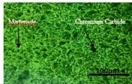
B: Carburizing surface heat treatment
