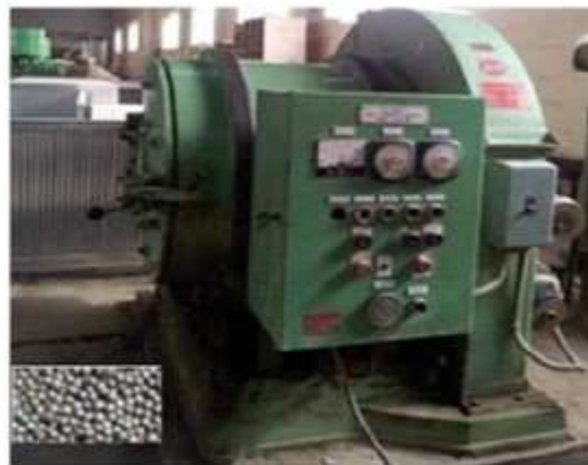
Figure 1: Shows the shot peening device with shot balls used.
